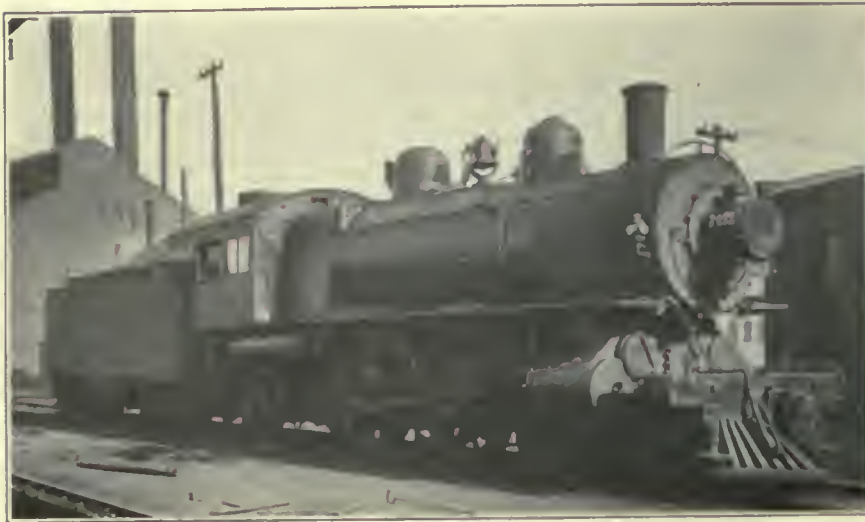
FIG. 378. LOCOMOTIVES. Passenger Locomotive of the Atlantic Type. Pittsburgh, Fort Wayne & Chicago Railway.
